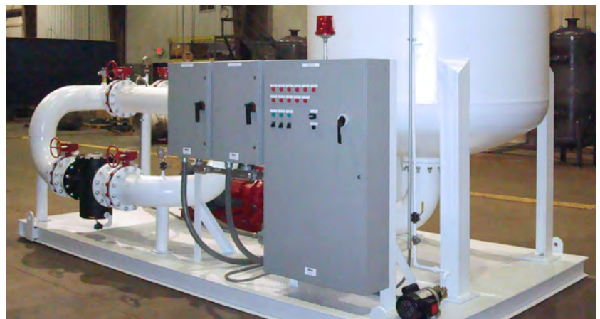
Internal and external piping is typically assembled during the final stage of production along with any required system testing prior to finishing.
