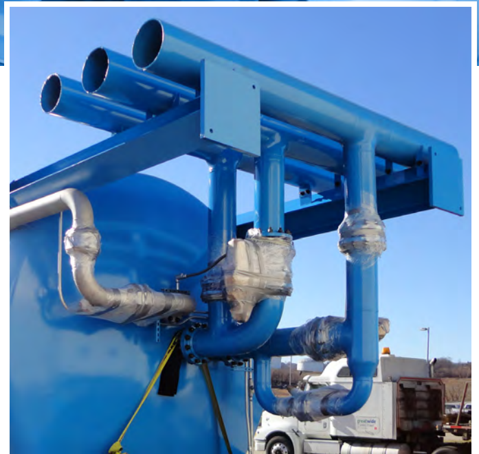
Internal and external piping is typically assembled during the final stage of production along with any required system testing prior to finishing.
